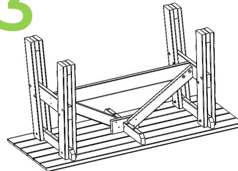
1º - APÓS TER ENCAIXADO TODOS OS PARAFUSOS, DAR UMA LEVE BATIDA COM UM MARTELO NA CABEÇA DO PARAFUSO E COM A CHAVE DE APERTO (FORNECIDA NO KIT) APERTAR TODAS AS PORCAS.
